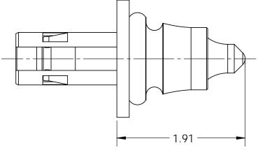
FULLY INSERTED INTO BORE OF HOLDER
